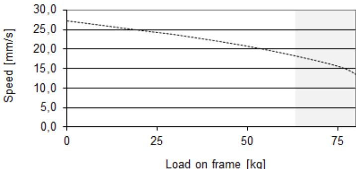
Above curve applies to a centrally placed load and is only valid in respect of duty cycle: 10% by 50% of max. working load or max. 2 min. continuously.
