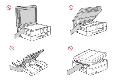
DO NOT touch the edges of the metal parts behind the rollers in the grey shaded area shown in the illustration. These parts have sharp edges and touching the metal parts behind the rollers may cut your fingers or otherwise injure them.
