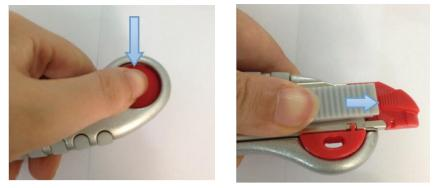
2.put snap off block hole on the first line of the blade, close the snap off line
