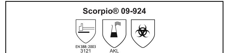
is in conformity with the provisions of the Council Directive 89/686/EEC and with the European harmonised standards EN420:2003+A1:2009, EN388: 2003, EN374: 2003, and is identical to the PPE which is subject to the EC Type Examination certificate number 03213528 issued by the Notified Body:
