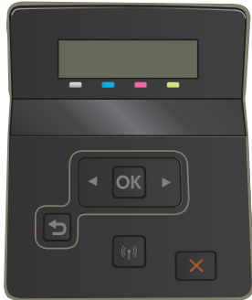
1 2-line control panel
