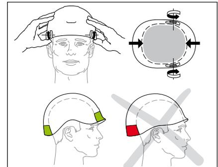
CenterFit adjustment system: The two adjustment wheels act simultaneously to adjust the headband and keep the helmet centered on the head. Adjustment wheels can be manipulated while wearing gloves.
