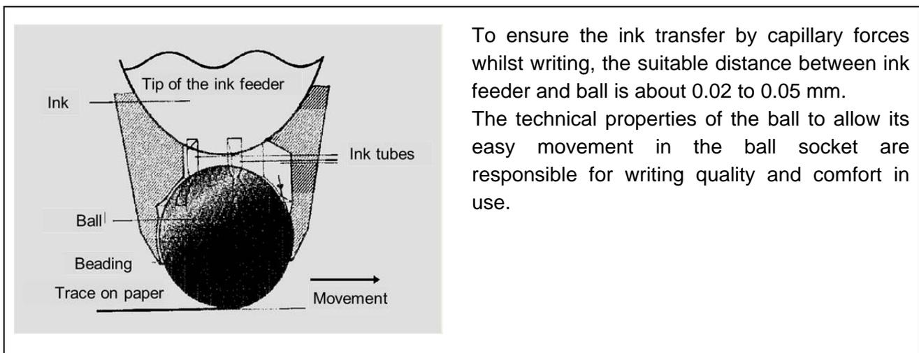
To ensure the ink transfer by capillary forces whilst writing, the suitable distance between ink feeder and ball is about 0.02 to 0.05 mm. The technical properties of the ball to allow its easy movement in the ball socket are responsible for writing quality and comfort in use.
