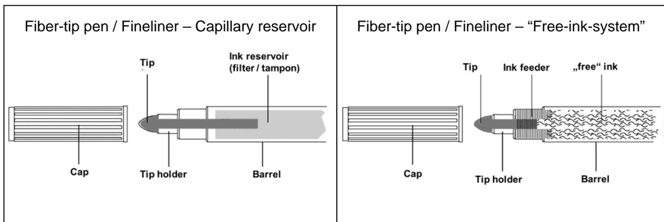
Writing instruments/marker pens designed without an ink reservoir use a complex ink feeder system combined with a tip to release a defined amount of ink on paper. A release of ink, e.g. by dropping or squirting or emitting to the environment does not take place.
