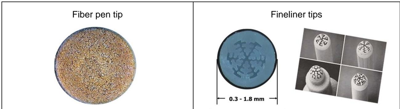
Fiber-tip pens typically contain 1.5 to 2 ml ink (~ 20% of pen weight). This correlates with a writing length of about 500 m (trace on paper) and thus would lead to an **application of 4 µl per meter**. Marking pens typically contain 5 ml ink (~ 20% of pen weight). This correlates with a writing length of about 500 m (trace on paper) and thus would result in an **application of 10 µl per meter**.
