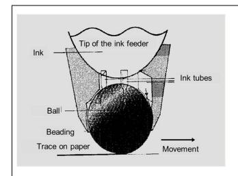
To ensure the ink transfer by capillary forces whilst writing, the suitable distance between ink feeder and ball is about 0.02 to 0.05 mm.
