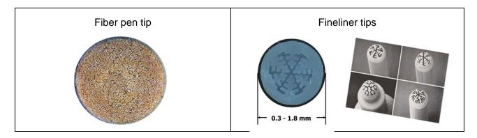
Fiber-tip pens typically contain 1.5 to 2 ml ink (~ 20% of pen weight). This correlates with a writing length of about 500 m (trace on paper) and thus would lead to an **application of 4 µl per meter**. Marking pens typically contain 5 ml ink (~ 20% of pen weight). This correlates with a writing length of about 500 m (trace on paper) and thus would result in an **application of 10 µl per meter**.
