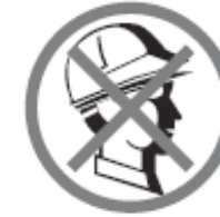
Incorrect — ball cap worn under hard hat
