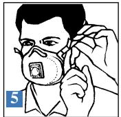
Strap tension may be decreased without removing respirator from the head by pushing out on the back of the buckles.
