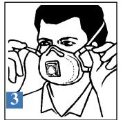
Adjust tension by pulling tabs of each strap, as shown.
