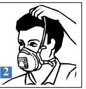
Place the top elastic strap around the head, above the ears. Untwist the strap.
