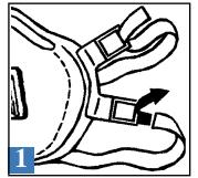
Thread top elastic strap through top buckles. Repeat for bottom strap and buckles. Place the bottom elastic strap around the head just below the ears. Untwist the strap.
