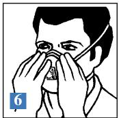
The seal of respirator on the face should be fit-checked prior to wearing in the work area. (a) Cover the front of the respirator with both hands, being careful not to disturb the position of respirator. (b) Inhale sharply. A negative pressure should be felt inside respirator. If any leakage is detected, adjust position of respirator and/or tension of strap. Retest the seal. Repeat the procedure until the respirator is sealed properly.
