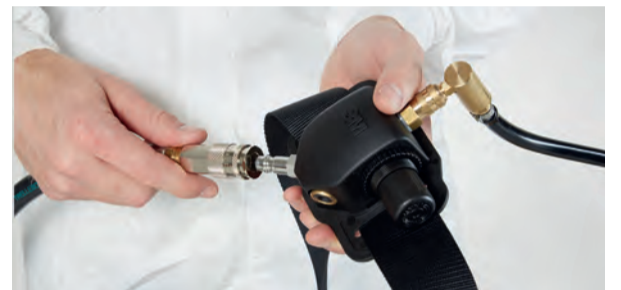
f | Connect the regulator up to a source of breathable quality supplied air. The inlet pressure should be set to between 3.0-7.0 Bar.
