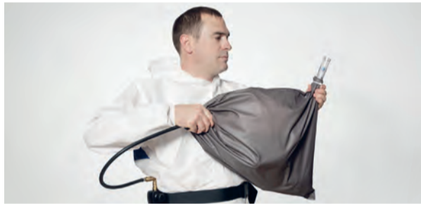
a | Set the regulator to the lowest flow setting using the adjustment knob and carry out an airflow check (minimum flow = 120 litres per minute). Ensure that a good seal is formed around the opening in the bag whilst performing the check.
